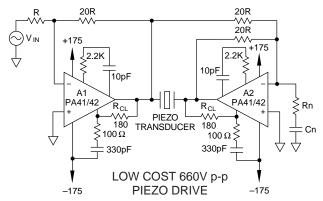
Two PA41/42 amplifiers operated as a bridge driver for a piezo transducer provides a low cost 660 volt total drive capability. The  $R_{\rm N}$   $C_{\rm N}$  network serves to raise the apparent gain of A2 at high frequencies. If  $R_{\rm N}$  is set equal to R the amplifiers can be compensated identically and will have matching bandwidths.
