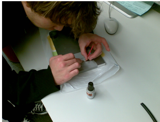
Figure 9: Glueing the wire onto the sample.
