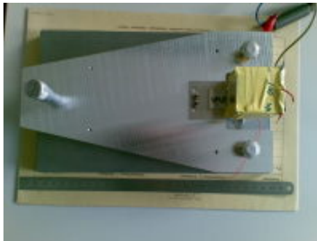
Figure 11: The provisional amplifier mounted onto the STM for testing purpose.
