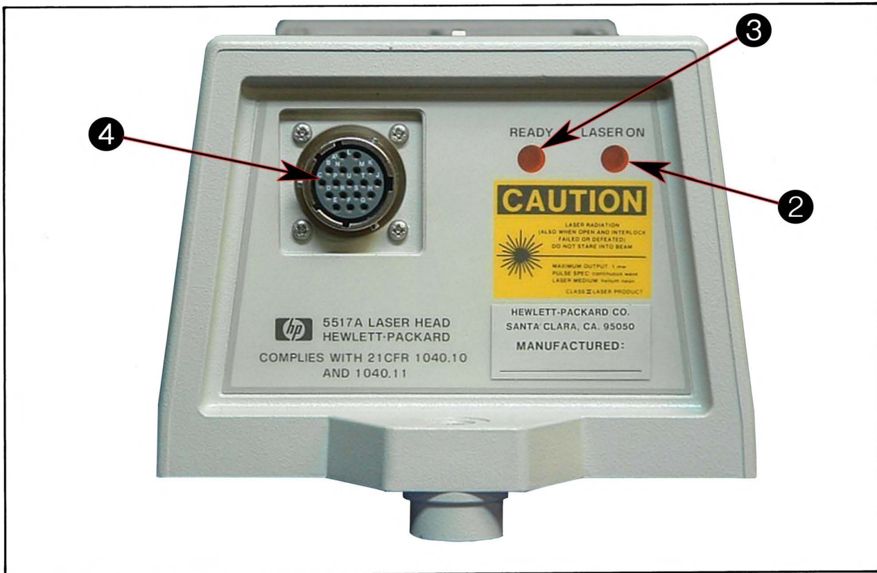
Figure 3-2. 5517A Laser Head, Rear Panel Connectors and Indicators
